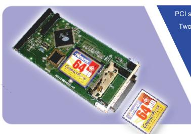
PCI single chip IDE controller (CMD PCI-648).
