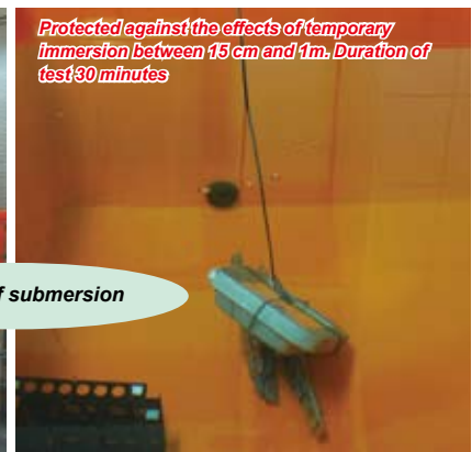
Test for protection against Water
