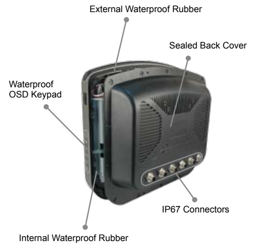
Protected against the effects of temporary immersion between 15 cm and 1m. Duration of test 30 minutes
